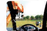
4 INCREASED VISIBILITY Bigger size front windshield and re-routing of hoses provide much better front visibility.
