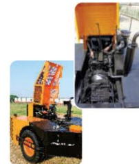
7 EASY MAINTENANCE The engine is easily accessible for daily maintenance checks including battery, air filter, oil dipstick and cooling system
